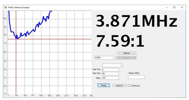
9:1 Unun, 470 ohms on antenna side. (Note that the software got confused because it isn't calculating the absolute value – it is really about 1.3:1 around 20 MHz)
