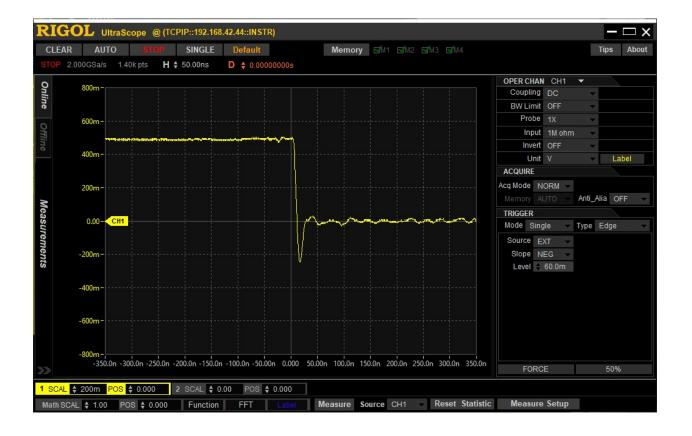
Next, I add signal pDBIN on channel 2 (pin 78 - the general read strobe) on channel 2. Channel 1 is still TMAXPU and the external trigger is negative going on TMAXPU, as before. We can see that pDBIN goes active 100ns before TMAXPU:
