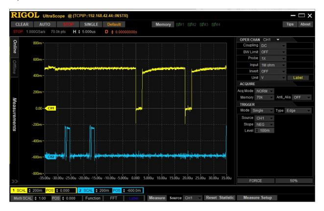
Here are a couple of traces on a much longer timebase (25us). The first was at a different spot in the code. The second is from the output to E001. There is clearly no danger of overlap between enabling the PDP11 output buffers (active low, CH1, also the trigger) and pDBIN (active high, CH2).
