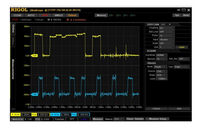
Finally, here is a trace with A3 and A11. My hope is that if I include some of the high order address lines in the equation (even though they should be the same as the low order address lines, as the ZPU board is jumpered to mirror I/O addresses) it will be less prone to the issue. (The trigger is back to TMAXPU).
