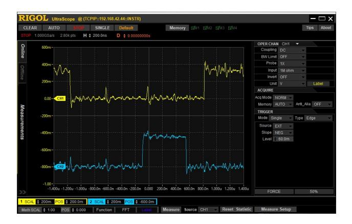
And here is A3 at the output of the 74LS244, triggered on TMAXPU, which shows a clear brief "glitch" on A3 in TTL "no man's land" that is enough for the CPLD to treat it as a 1. So, the closer I get to the CPLD input, the worse it looks.
