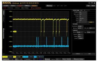
I then removed the term !bpWR from the equations for !OE\_C, !OE\_D and !OE\_B (it was not present for OE\_A, which is a read cycle). I have not removed it from bsXTRQ. Here is what it looked like. CH1 is S100 pWR\* and CH2 is the data on pin13 of U20. Note the little positive excursion that happens in the data initially. That matters not at all – it is during the time when the data has not yet been set up by the J11:
