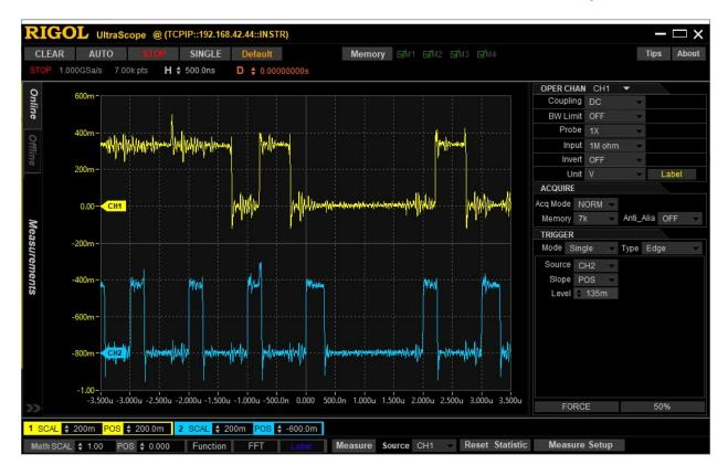
Here is a *typical* console input loop waveform using John Monohan's Z80 board, without the PDP11V2 board. Note that there is somewhat less noise on the address lines – but there is still some present, consistent with the observation that the false activation of the PDP11V2 board happens less often with this CPU board – but does still occur (though there is not any indication of spike on A3 sufficient to be a trigger.)
