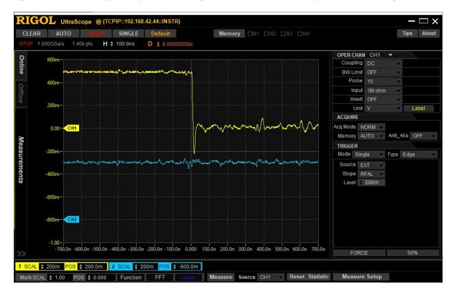
So, I paralleled the 0.1uf caps on the back side, but that did help. Neither did 10uf. Nor did a .01uf. The 8v line also has a corresponding drop. The drop is about 10ns long (so, about 100Mhz), so no wonder adding 10uf did not make any difference. Later I tried adding .0047 and an additional 10uf at the regulator. That actually turned it into a little positive going bump – but the board still activated.
