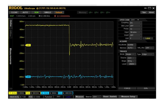
So, I then added a "probe point" on pin 8 of U21, the 74LS07 that generates the signal fed to U25. It (CH2) is just *barely* reaching into the 0.8v "no man's land". The CPLD is being very very touchy. Interestingly, the j0,efff command *does* do I/O – it checks for the operator pressing ESC to terminate the test. Curiously, if I put a probe point right on U25's pin, the problem disappears completely.
