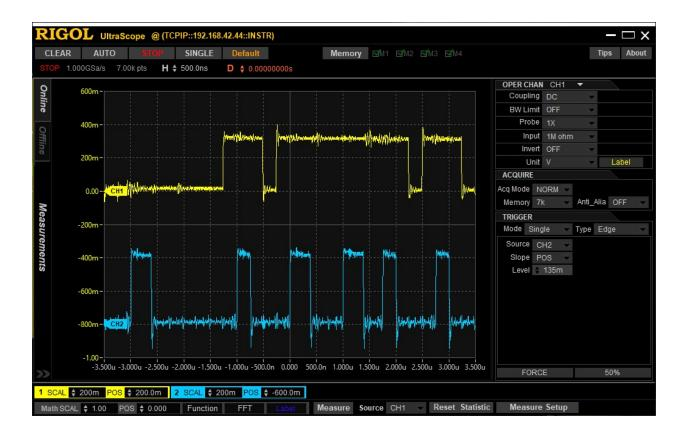
This picture is the *typical* console wait loop with the ZPU back in the system, and a Godbout active bus terminator at the end of the bus. There is considerably less noise, but the address line spikes are still present. (Especially notable is the one towards the right of the trace). Trigger is Ch2 (pDBIN)
