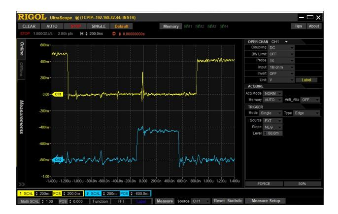
Note that this signal on A3 is not simply ringing – it is occurring when the signal is at 0 for an eternity (a full microsecond) before the problem. This is why adding termination did not help at all. It is happening roughly 100ns after pDBIN goes active, when nothing ought to really be going on anywhere.
