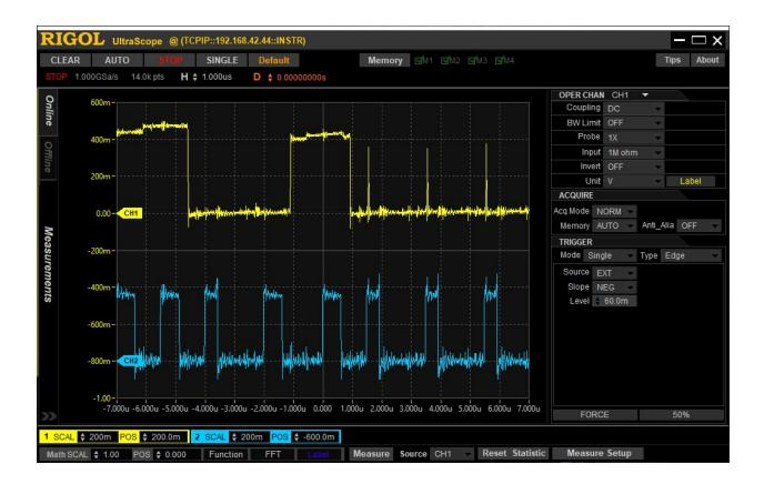
And here is the same sequence, but at the bus connector instead of at the output of the 74LS244 U30.
