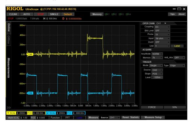
Here is a *typical* console input loop waveform using the ZPU without the PDP11V2 board. This waveform is taken at 4MHz to be consistent with the next one – but note that the earlier waveforms were taken at 2MHz. The ZPU is a good bit noisier than the newer Z80 board, below.
