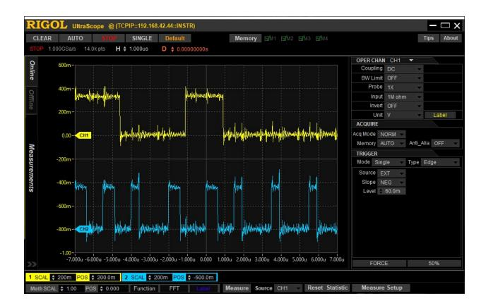
Here is a *typical* console input loop waveform (triggered on pDBIN) using the ZPU without the PDP11V2 board. As before, CH1 is A3, CH2 is pDBIN (which is also the trigger). This one was taken at 2MHz, as were the earlier waveforms:
