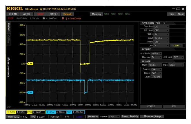
And here is the new signal compared to pDBIN (CH2). It shows no danger at all of this new signal causing bus contention by overlapping with pDBIN.
