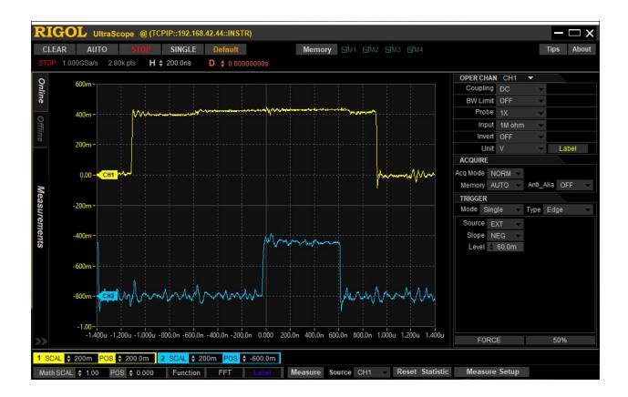
Here is the same sequence, but with a longer timebase (again the J11 is removed). It shows A3 at the 74LS244 output spiking during some, but not all, pDBIN cycles – and, if one looks carefully, it is always about 80-100ns after pDBIN goes active (yes, it is hard to see at this scale). The trigger was the same (TMAXPU), but in this case that was manually generated by command.
