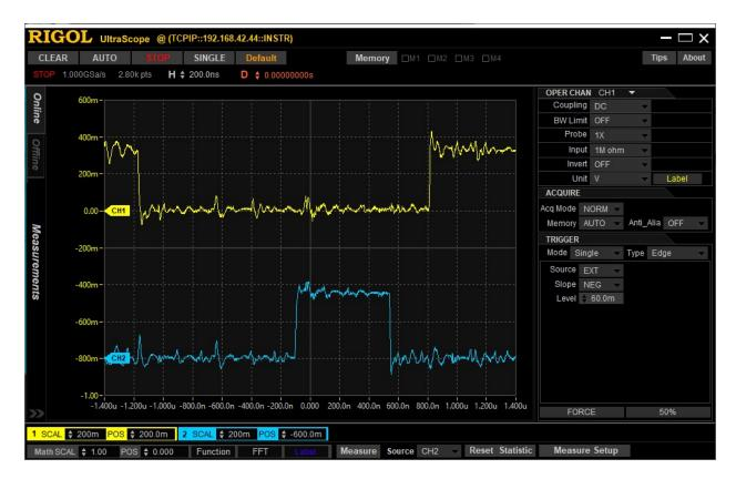
WTF? A3 is NOT really a 1. But it is marginally close to 0.80v (x10 attenuation on the probe) to be in "no man's land" for logic levels. A3 is driven on the Cromemco ZPU by IC25, a 74367 (as are most of the bus lines), and appears on the PDP11V2 card at U30 pin 12, a 75LS244 (U30 - soldered in place underneath the J11). I tried swapping 74367's and even swapping in an 8T97 – no difference. It is also worth noting that these blips in A3 are happening every 200 to 400 ns.
