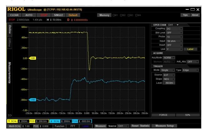
Next, I replace pDBIN with sINP. It is high – indicating an input I/O operation, as expected. I also lengthened the timebase to provide more context – but the trigger point is unchanged. So, sINP goes active about 700ns before TMAXPU, and pDBIN went active about 100ns before as well.
