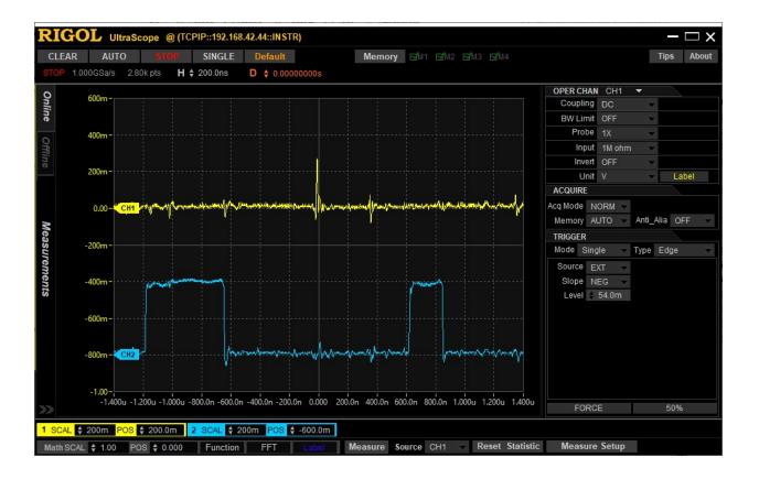
As a final check, I connected CH1 to the output of A3 on the 'LS244, and used the 'scope's "runt" trigger to capture the pulses (independently of TMAXPU), and displayed the input on CH2. (I also separately checked A11, and there were certainly times when A11 spiked as well.)
