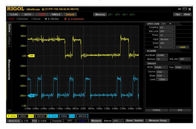
And here it is with the active terminator in place, with the ZPU at the output of the 74LS244, U30 (but not the same timing as above, of course), with the 2V+ spikes present. Trigger remains pDBIN.
