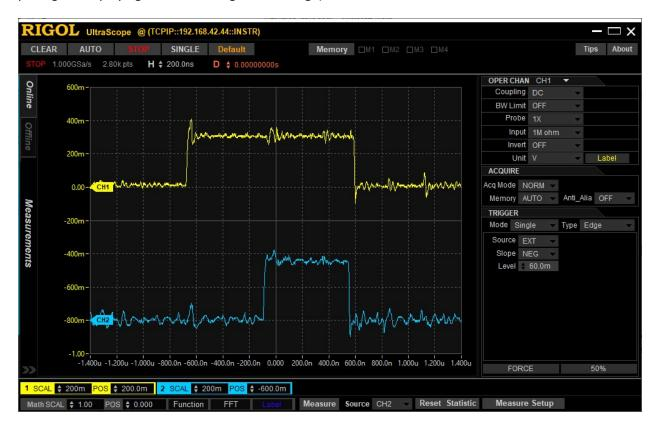
Since sINP is the later signal, I left that in place on channel 2, and picked an address line (A3) that it supposed to need to be a '1' in U25. The trigger is TMAXPU. The logic equation I use is this (because I have my Z80 set to mirror I/O addresses, I am only looking at the least significant 8 bits for 0xED):
