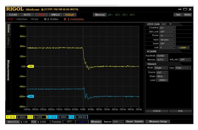
Finally, here is a picture of the Z80 outputting to the same port (the character is "A") (CH2). CH1 is the pWR\* signal for the I/O (pin 77). It comes slightly after the trigger, which is sOUT (pin 45).
