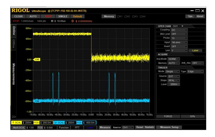
This made me a little suspicious. Could this be a noise immunity issue caused by noise on the +5V rail? So, I 'scoped the rail (with a probe point right at one of U25's bypass capacitors) during this new issue. Note the dip, of about 0.5v, right when this happens.
