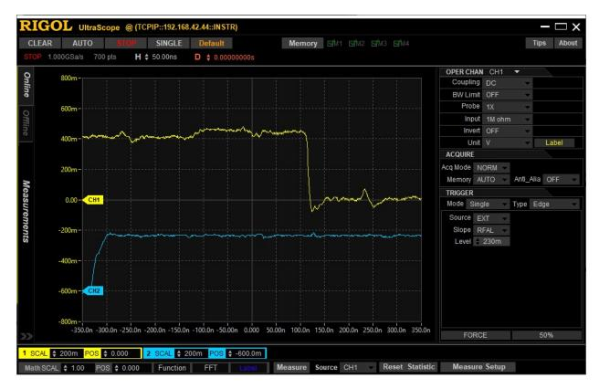
The idea I had is to remove the signal bpWR\* from the equation for OE\_C, OE\_D and OE\_B. Here is a trace of what that would look like. CH1 (and the trigger) is the proposed new signal. CH2 is the output data – plenty of setup time.
