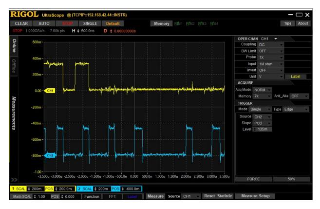
This picture of a *typical* console wait loop was taken with the PDP11V2 board back in place, the ZPU, with active termination. The noise on the address line is still apparent (note particularly the right hand side of the screen, where the spike occurs during the input cycle.) Trigger is pDBIN
