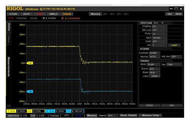
Here is the same setup, but with the active terminator removed. In this situation the correct output is observed, but that is likely simply because the data waveform has a baseline starting at 1.6v – closer to 0. pWR\* still has not given the data time to stabilize. It probably works only because of a couple of gate delays on the Propeller board give it just enough time.
