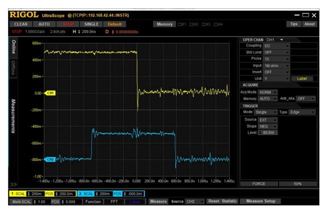
So next, I put up both sINP (bottom) and pDBIN (top) to show that relationship. The external trigger is still TMAXPU. Multiple captures demonstrated that TMAXPU is only triggering on an I/O operation (the console input loop, though sometimes it happens during the status polling for displaying the monitor sign-on message).
